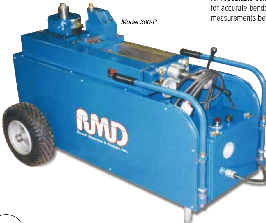
The Model 300 can accurately bend a wide range of materials to various angles up to 180°.
